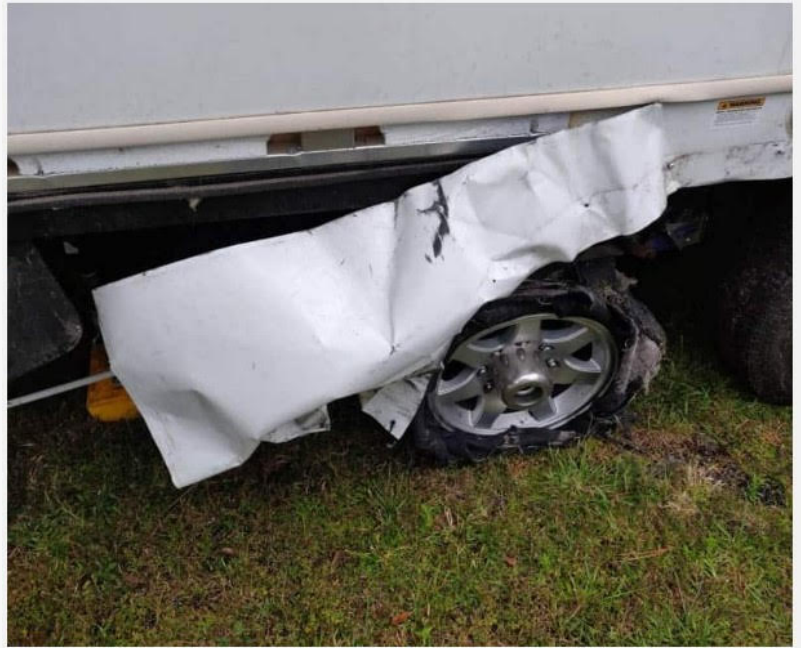
Typical Blowout Damage without RV-DE-FENDER example 2
