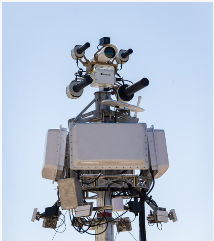
Sawtooth CUAS Layered Radar, EO/IR, and RF Sensors System with Defeat Capability
