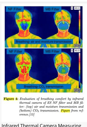
Infrared Thermal Camera Measuring Breathing Comfort for Electrospun Nanotechnology vs. Disposable Meltblown
