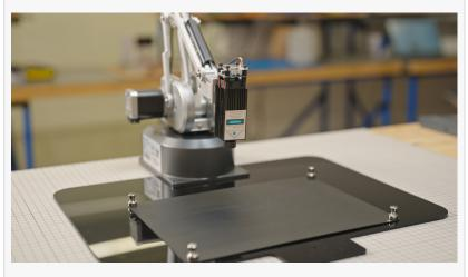
classic metal structure and occupies only an area of A5 paper. It is the first robotic arm equipped with a high-performance stepper motors of Elephant Robotics. It is stable and owns  $\pm 0.1$ mm repeated positioning accuracy. What's more, ultraArm comes with 5 kits together including slide rail, conveyor belt, and cameras.
