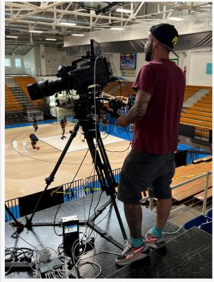
Dejero EnGo mobile transmitters blend cellular networks from multiple carriers so Quality did not have to rely solely on the venue's limited connectivity or send a satellite truck to the island
