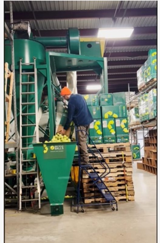
Processing tennis balls into the recycling machine
