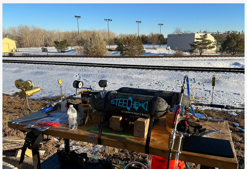
Pilot project using Steelhead Composites Pressure Accumulator to boost filling pressures at hydrogen filling stations
