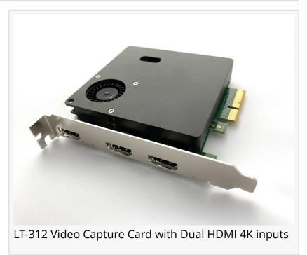
The LT-300 series includes overlay features for text, shape(s) and image injection with alpha blending, allowing customers to inject their own overlays and templates onto the incoming video streams and view this both on the HDMI direct out and via the host. Color space conversion and color adjustment are also provided. The product range is ideally suited to Medical, Aerospace, Industrial, Military and other real-time and high-reliability applications.
