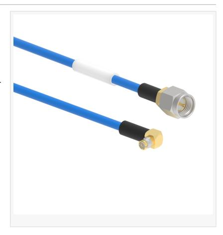
The SMA plug features a gold-plated, stainless steel anti-torque body while the SMP plug is manufactured with gold-plated, beryllium copper. The right-angle SMP also provides for a lower mated height with no bend radius for applications with small size requirements. This assembly offers excellent electrical performance up to 18 GHz and is available in multiple standard lengths.
