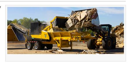
horsepower (399.7-kW) CAT C13B T4F/Stage V diesel engine, a Series III duplex drum, an aggressive infeed to accommodate a variety of materials, and many performance and durability features. It's quiet, too, with a working sound level of 112 decibels.
