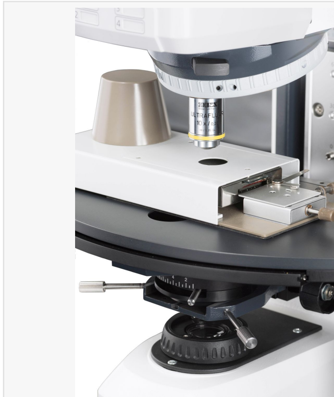
Measuring the refractive index of glass fragments with rIQ 2.0
