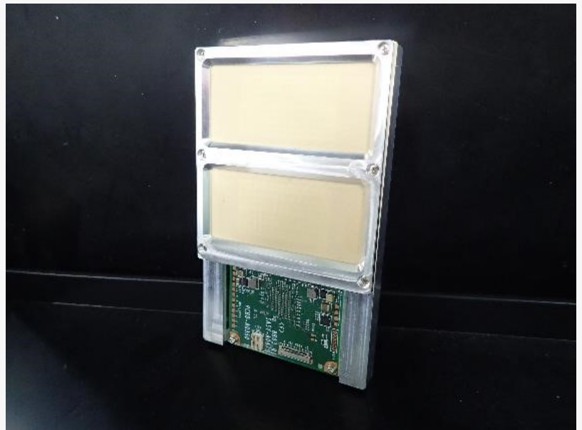
60 GHz millimeter-wave wireless communication module high sensitivity version
