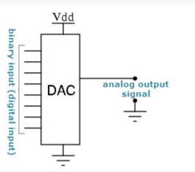
DAC mainly consists of a digital register, an analog electronic switch, a bit power network, a summing operational amplifier and a reference voltage source (or a constant current source).
