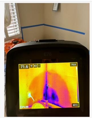
Using thermal imaging we can see how far the moisture has spread.
