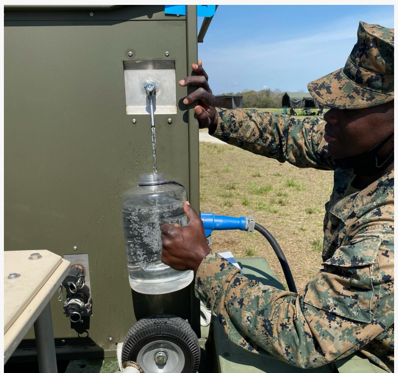
RussKap Water's OASIS Atmospheric Water Generator (200 gallons/day) dispensing clean drinking water made from the air.
