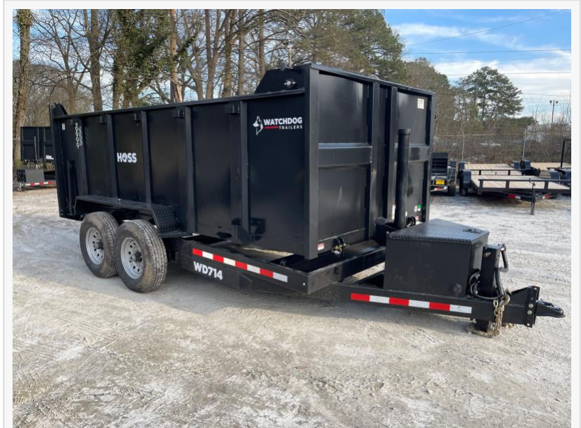
7x14 Dump Trailer With 4' Sides & Telescopic Lift Cylinder
