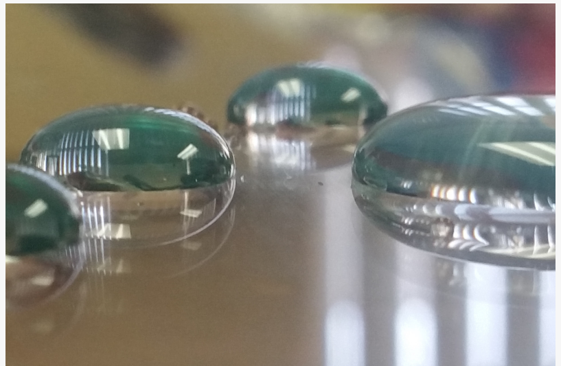
Water drops on glass that was treated with DiamonizeXP by Diamond Seal Systems
