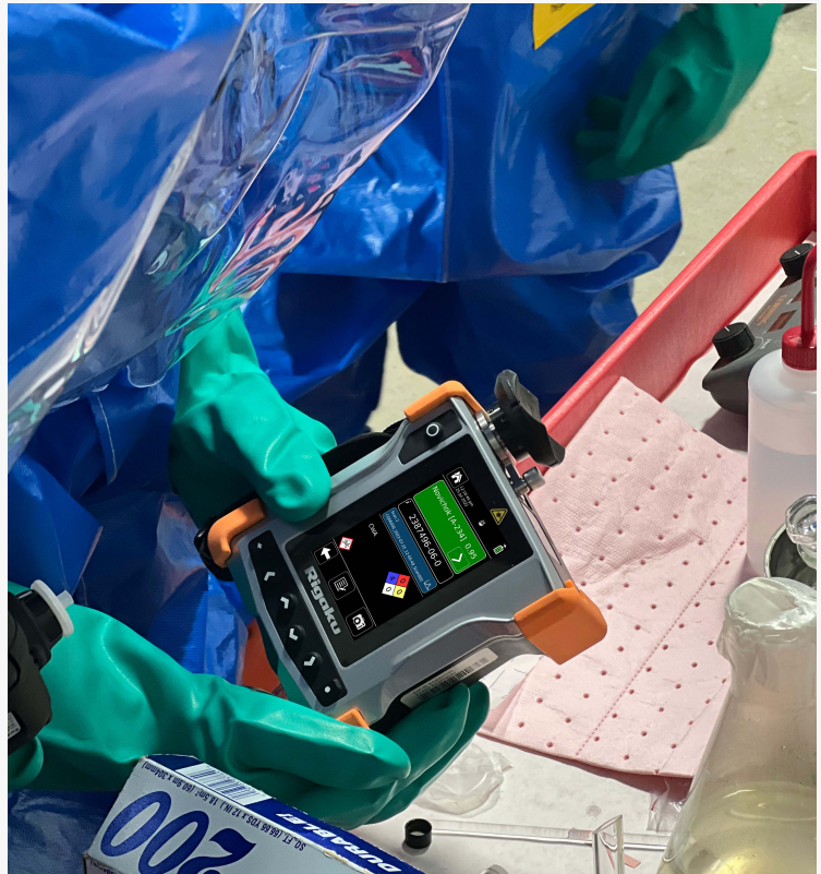
Rigaku ResQ CQL handheld 1064 nm Raman analyzing Novichok chemical weapon.
