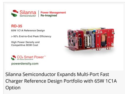
rapidly. Built around Silanna's CO2 Smart Power™ advanced AC/DC controller and high-frequency DC/DC converter technology and featuring a superjunction FET, the RD-35 simplifies and speeds the development of low-energy consumption multi-port 65W fast chargers offering USB Type-A and Type-C functionality.
