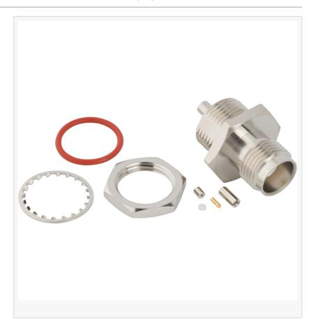
These TNC connectors are constructed with brass bodies and hardware that are nickel plated, along with brass and beryllium copper contacts that are gold-plated. Their front mount configuration makes them tamper-resistant which is useful in systems that are located outdoors or in harsh environments. These connectors are suited for WiFi 6, outdoor and remote antennas and smart application connectivity.
