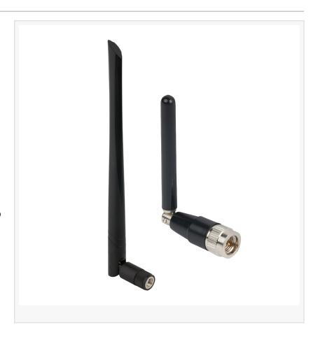
External antennas have a number of design options – straight and swivel whip-style, and panel and external mount cabled designs. They are constructed from common RF interface materials with plastic antenna casings and mechanical hinges and swivels. These antennas are often mounted on the outside of a device by means of an RF connector interface. They are made for indoor and outdoor use with robust designs available for harsher environments.
