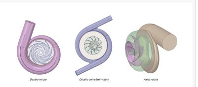
Support for Double volute for pumps, Double entry volutes for turbines or compressors and Axial volutes for chillers or rocket applications.
