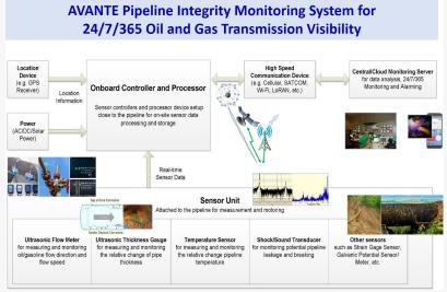
Sensor-based Autonomous Pipeline Integrity Monitoring System for Predictive maintenance analysis and Timely Alerts of Exceptions for Remedial Actions
