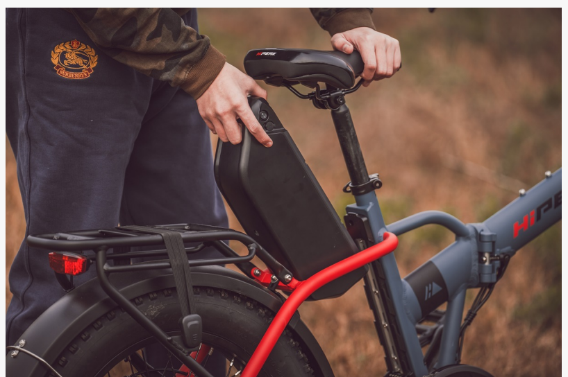
48V 15Ah Removable E-bike Battery
