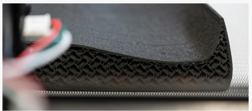
One Pro 3D belt printer producing orthopedic insole with structured infill for individual density
