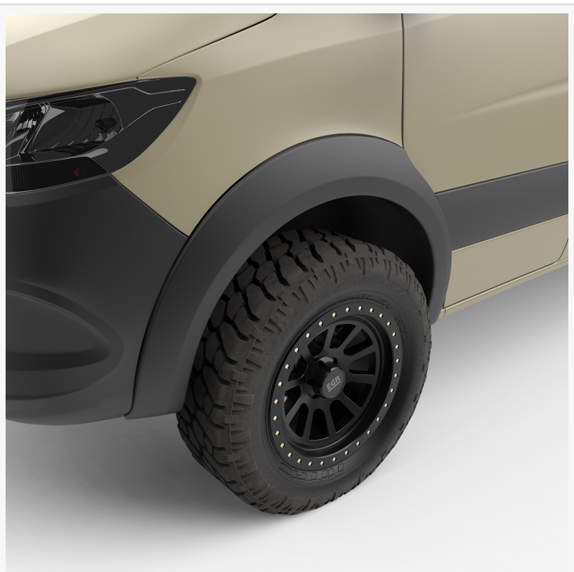
Close-up of EGR USA's Rugged Fender Flare installed on a Mercedes-Benz Sprinter Van
