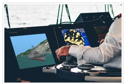
SPx Video Simulator can be combined with SPx Radar Simulator to build and test systems that use both cameras and radars.
