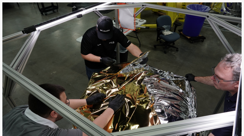
installation of multi-layer installation
