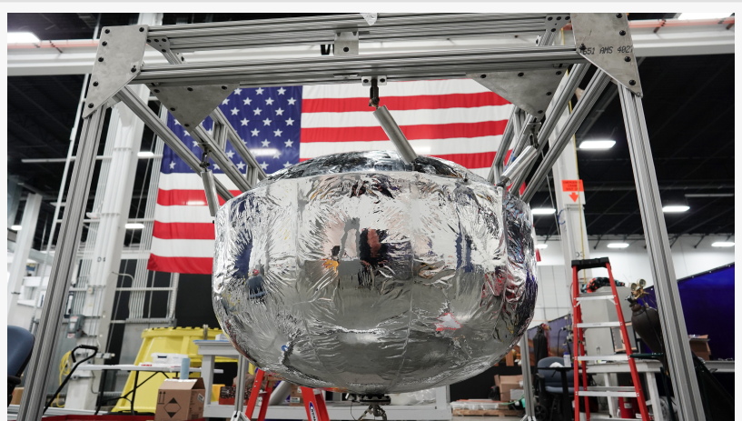
Composite liner-less tank in the process of receiving thermal wrap.
