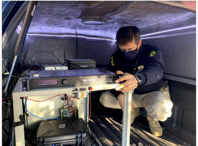
A Dejero GateWay M6E6 network aggregation device was installed inside the Polícia Rodoviária Federal Mobile Command Vehicle
