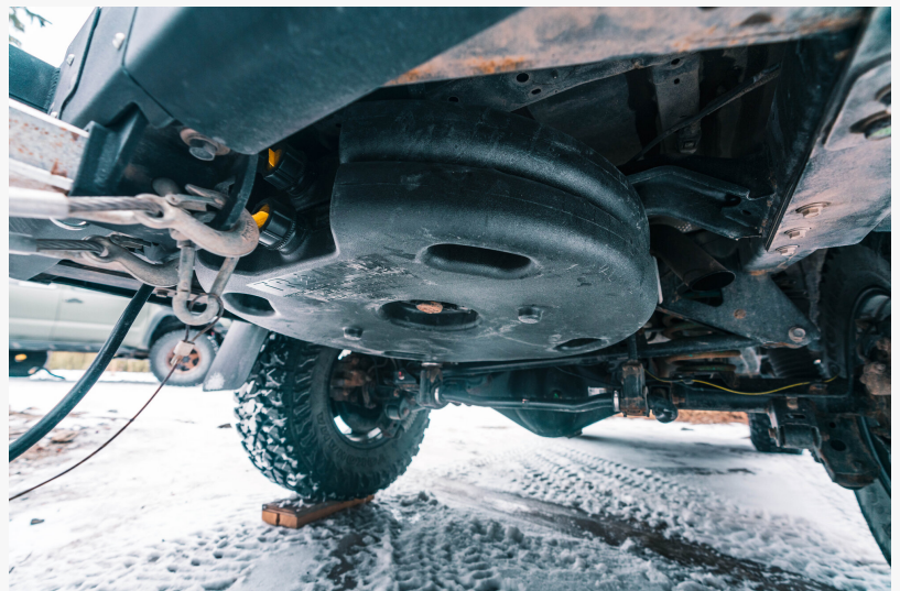
Trail'd Tank Installed
