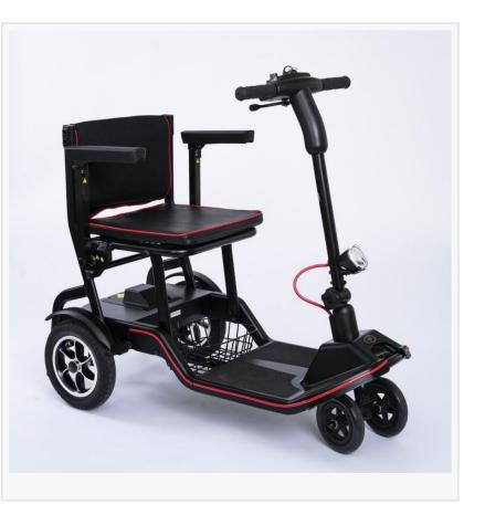
As a testament to its dedication to user safety, Feather Mobility has equipped the Featherweight Electric Scooter with puncture-resistant tires, a responsive electromagnetic braking system, and bright LED headlights and taillights for enhanced visibility during both day and nighttime use.
