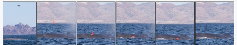
Photo sequence of a UAV deploying a DTag on a blue whale
