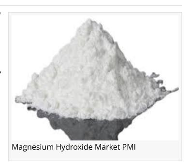
One of the major applications of Magnesium Hydroxide is as a flame retardant material. It is used in a variety of products such as plastics, rubber, textiles, and coatings to improve their fire resistance properties. Magnesium Hydroxide releases water when heated, which helps to cool down the temperature of the surrounding area, preventing the spread of flames.
