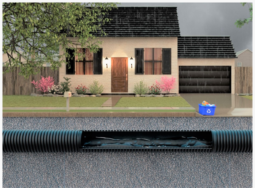
Recycled material is being used to make corrugated HDPE pipe for stormwater drainage.
