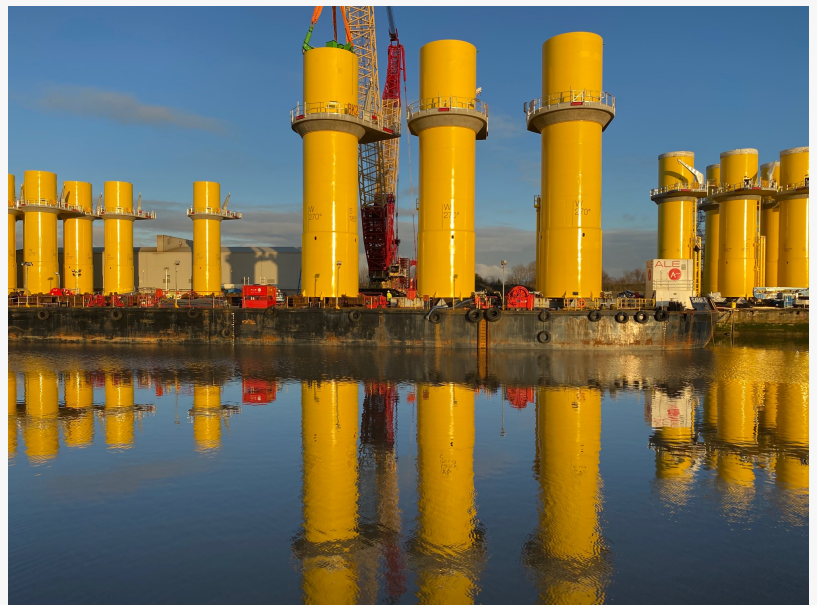
Transition pieces destined for Borssele offshore windfarm located near Belgium and the Netherlands
