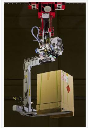
This robotic system is capable of handling cargo of a variety of sizes and weights, even odd-shaped cargo.
