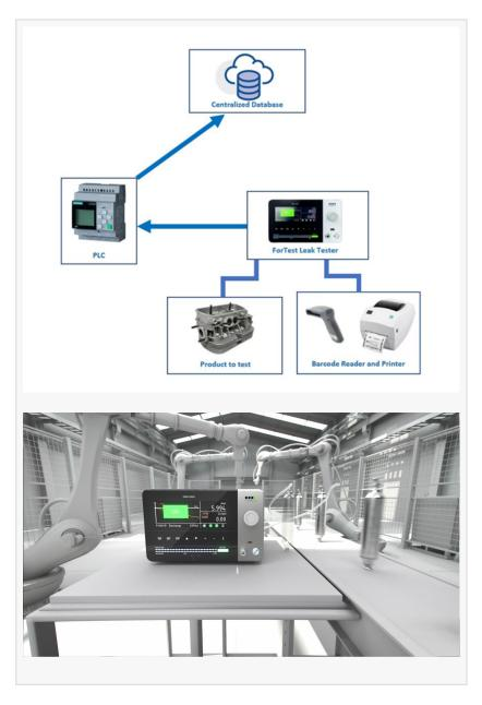
ForTest also provides support for standard industrial protocols, such as Modbus, Profinet, Ethernet IP, Ethercat and soon also OPC UA, allowing ForTest equipment to communicate with almost any device on the market, for example PLC and PC.
