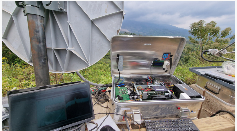
Fig. 1: The electronic system is housed in a metal box to prevent it from humidity, rain and wildlife in the jungle
