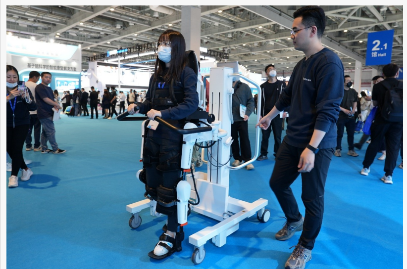
ExoMotus™ M4 Lower Limb Exoskeleton with integrated balancing support frame for gait training.
