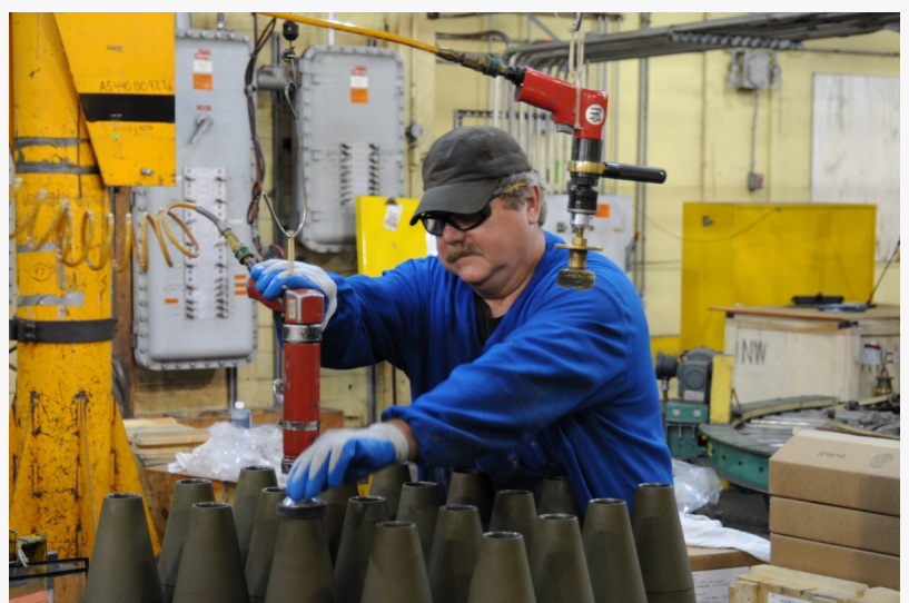
A contractor employee at Iowa Army Ammunition Plant performs a load, assemble and pack operation on a 155mm artillery round. (U.S. Army Photo, Iowa Army Ammunition Plant)
