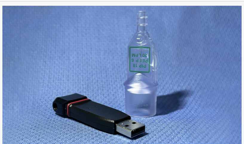
A USB flash drive (front) next to the HOPE inVent, 3D printed miniature ventilator. Credit: William Pritchard, Clinical Center, NIH
