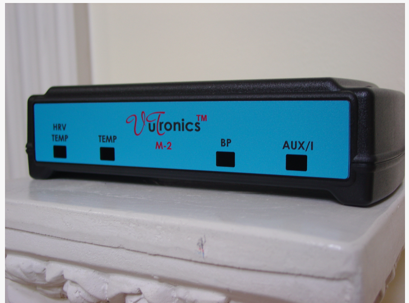
Wireless Data Acquisition System
