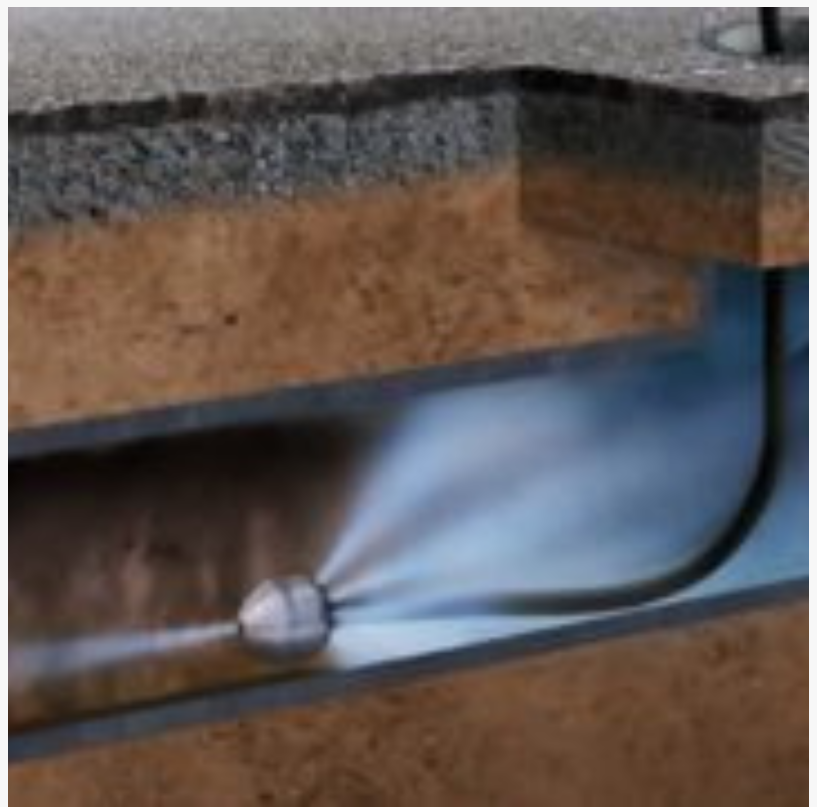
The drain must be thoroughly cleaned before installing the drain lining.
