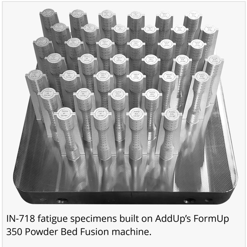
IN-718 fatigue specimens built on AddUp's FormUp 350 Powder Bed Fusion machine.
