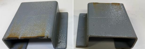
**FBE coated edges corrode quickly upon exposure to 5% salt water. The corrosion quickly propagated outward to other areas.**
