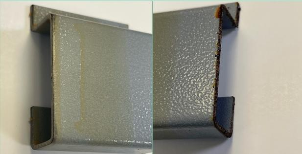
**Cut edge coated with FLUOROSEAL® CPC-EXT-7280 shows no sign of corrosion**
