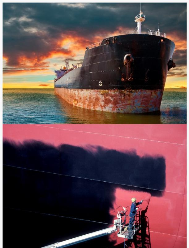
FLUOROSEAL® crosslinked PVDF corrosion protection coating is a single component, roller, brush and spray coating that is dry to the touch in hours and can be put into service in 2-3 days. A thin 30-50micron coating thickness is adequate when used as topco
