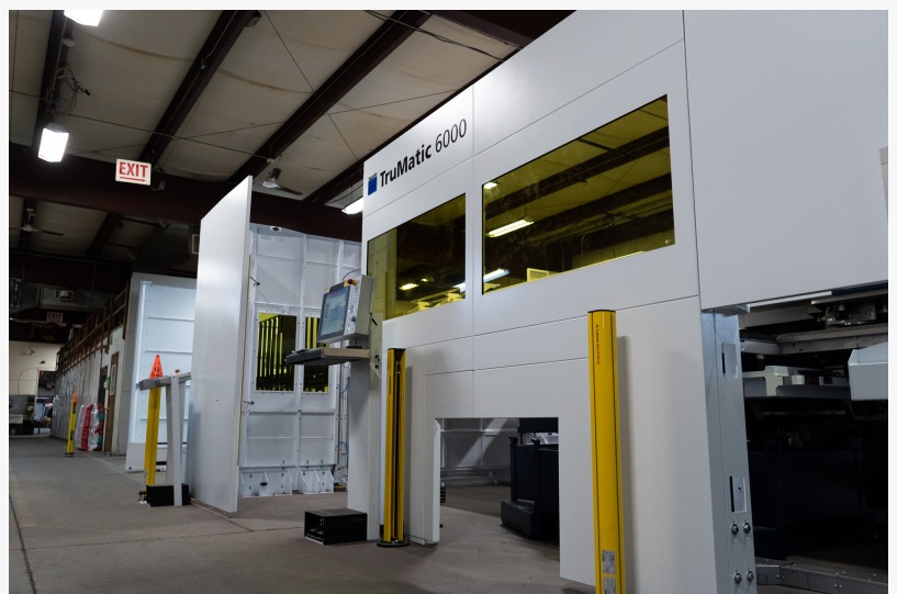
Chapco, inc. Chester, CT - New Trumatic 6000 fiber laser and punch combo work center
