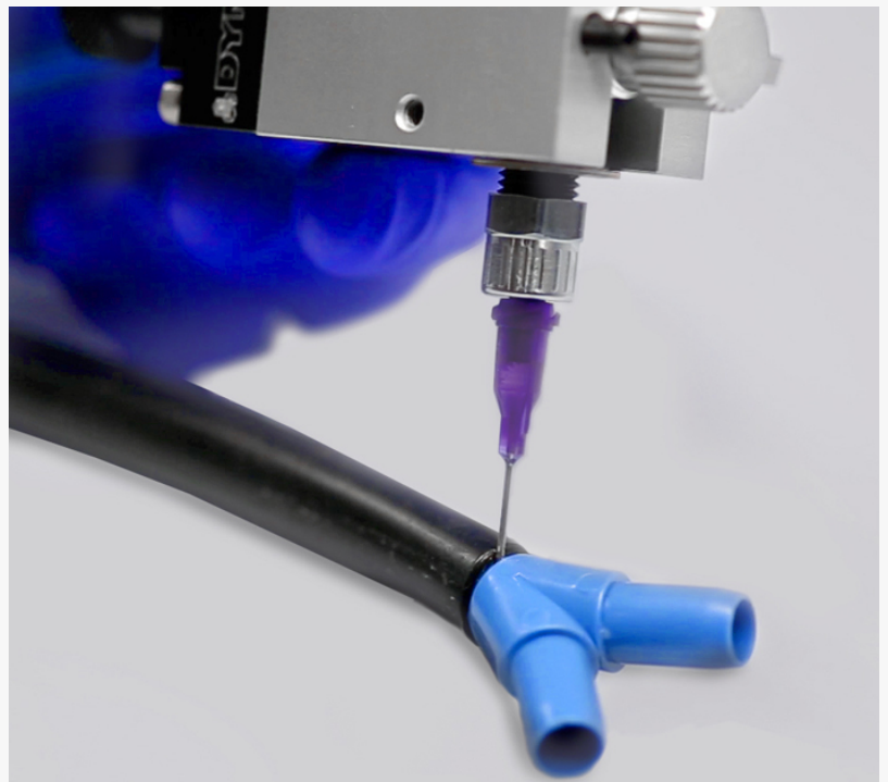
A Dymax Hybrid Light-Curable Adhesive is Dispensed onto Substrates
