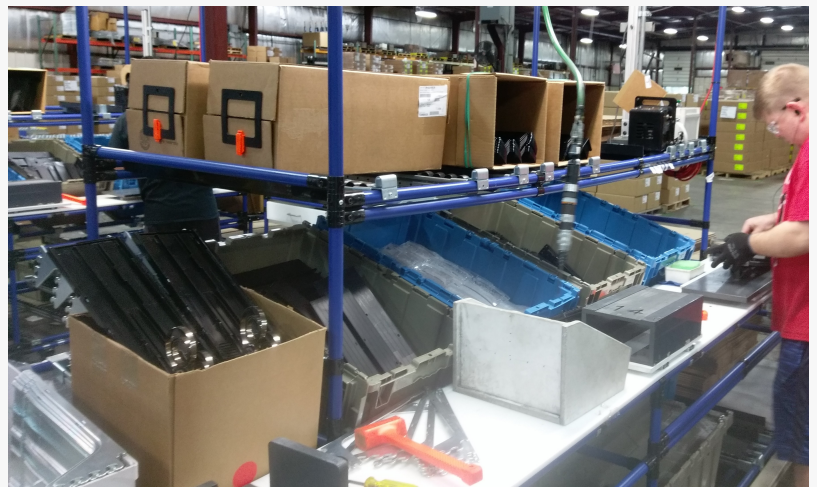
Collapsible end-loading corrugated boxes at an assembly cell
