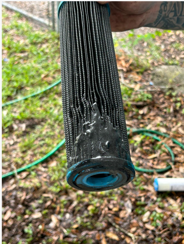
Sediment filter- Needing replacement & service- Lakewood Park
