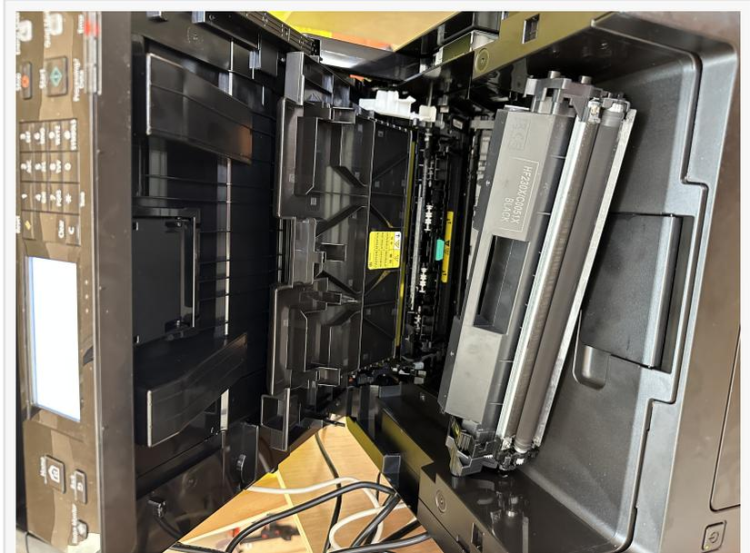
Converting standard laser printer to electrode and graphene printing
